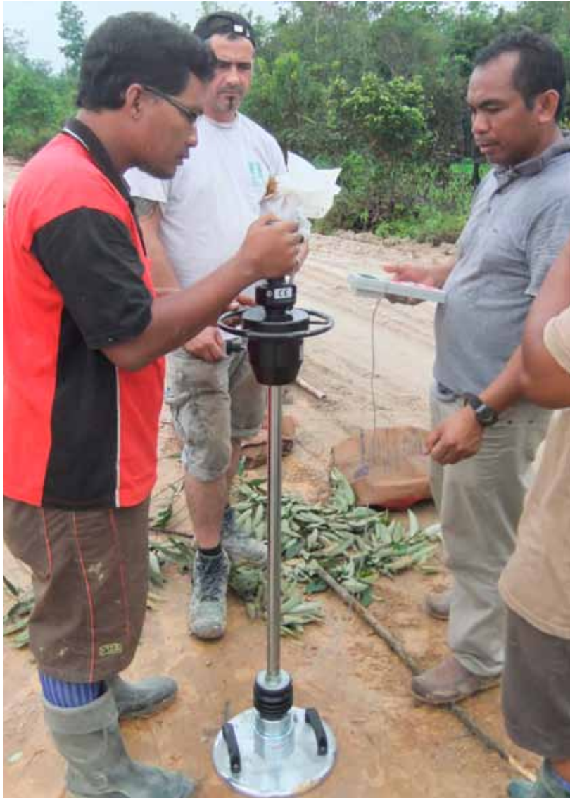
Analyse of the load bearing capacity by using a dynamic falling weight drop tester
