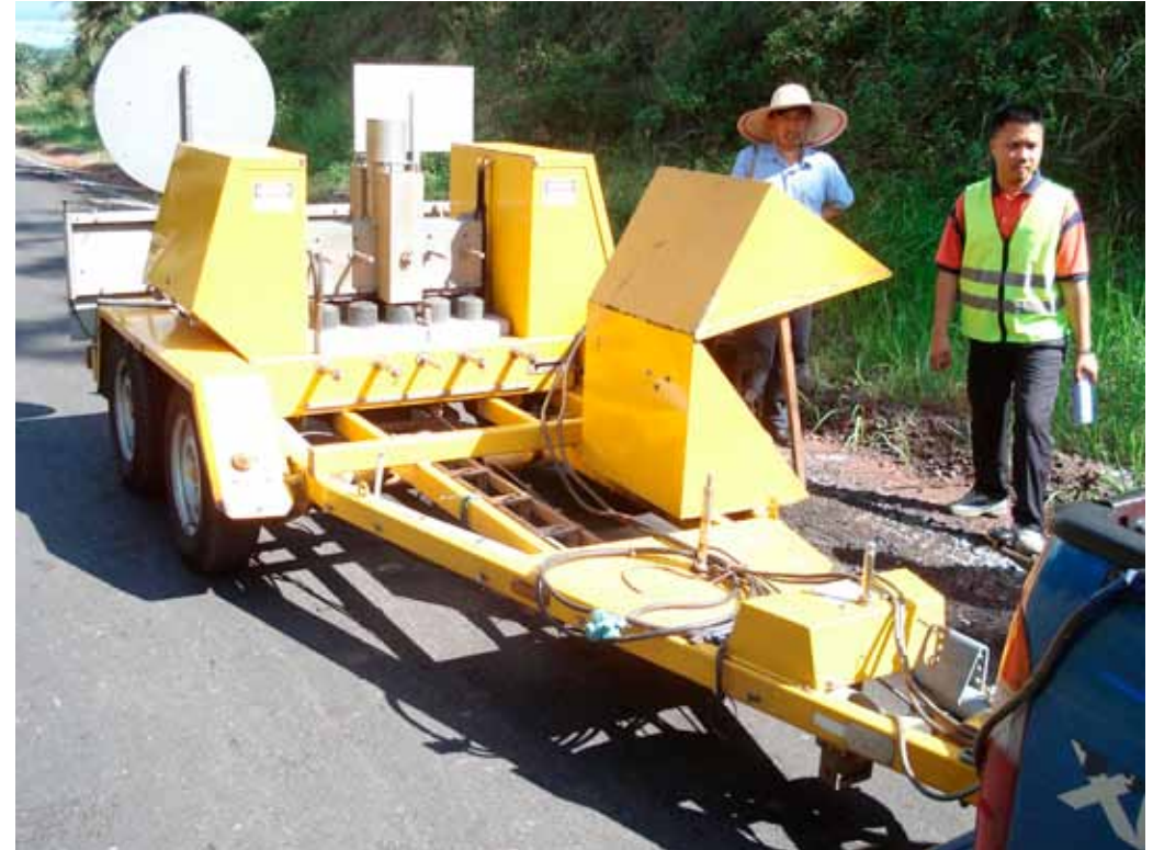
Fig 9: Bearing capacity measuring by means of a falling weight deflectometer (FED) on the road covered with an asphalt course of 5cm.
